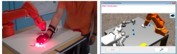
Fig. 1. (Left) Snapshot of human-robot task execution from human subject experiments, (Right) RobotStudio® point-and-click simulation environment for robot training used in our prior investigation.
