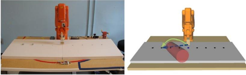
*Figure 1.* Illustration of human-aware motion planning. The left panel depicts a shared workspace in which a human and robot are placing and sealing screws, respectively. The right panel depicts both the standard, shortest-path motion (dashed arrow) and a human-aware motion (solid arrow) that the robot could take given the expected human workspace occupancy, represented by the cylinder.
